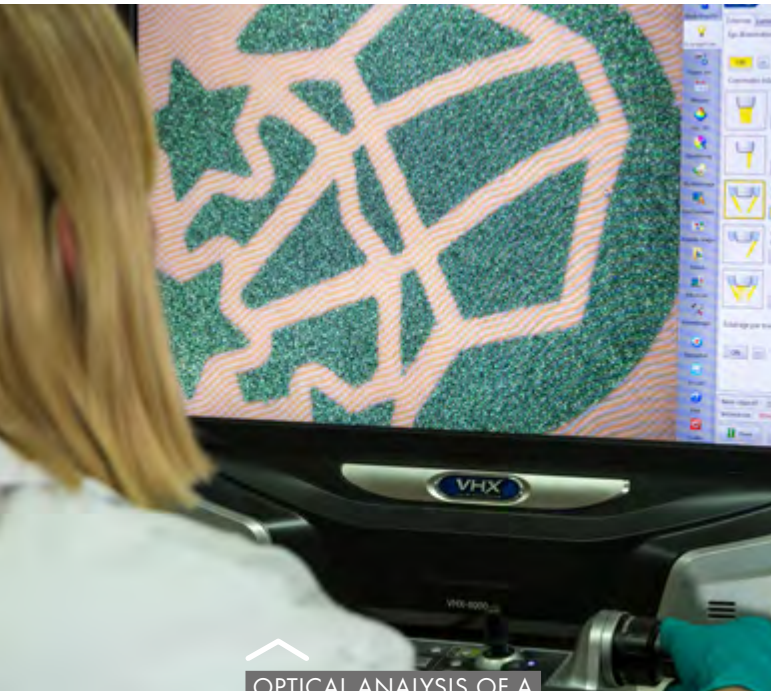
OPTICAL ANALYSIS OF A SECURITY FEATURE.
