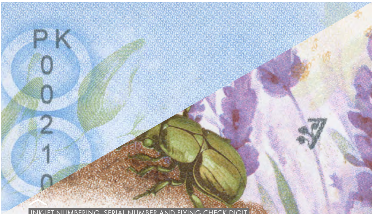
INK-JET NUMBERING, SERIAL NUMBER AND FLYING CHECK DIGIT
