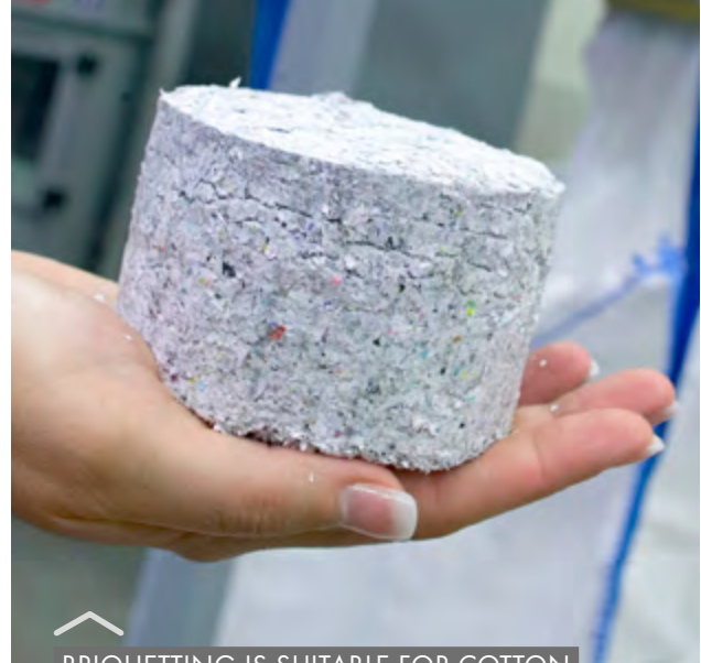
BRIQUETTING IS SUITABLE FOR COTTON SHREDS, CAPACITY UP TO 1,200 KG/HR
