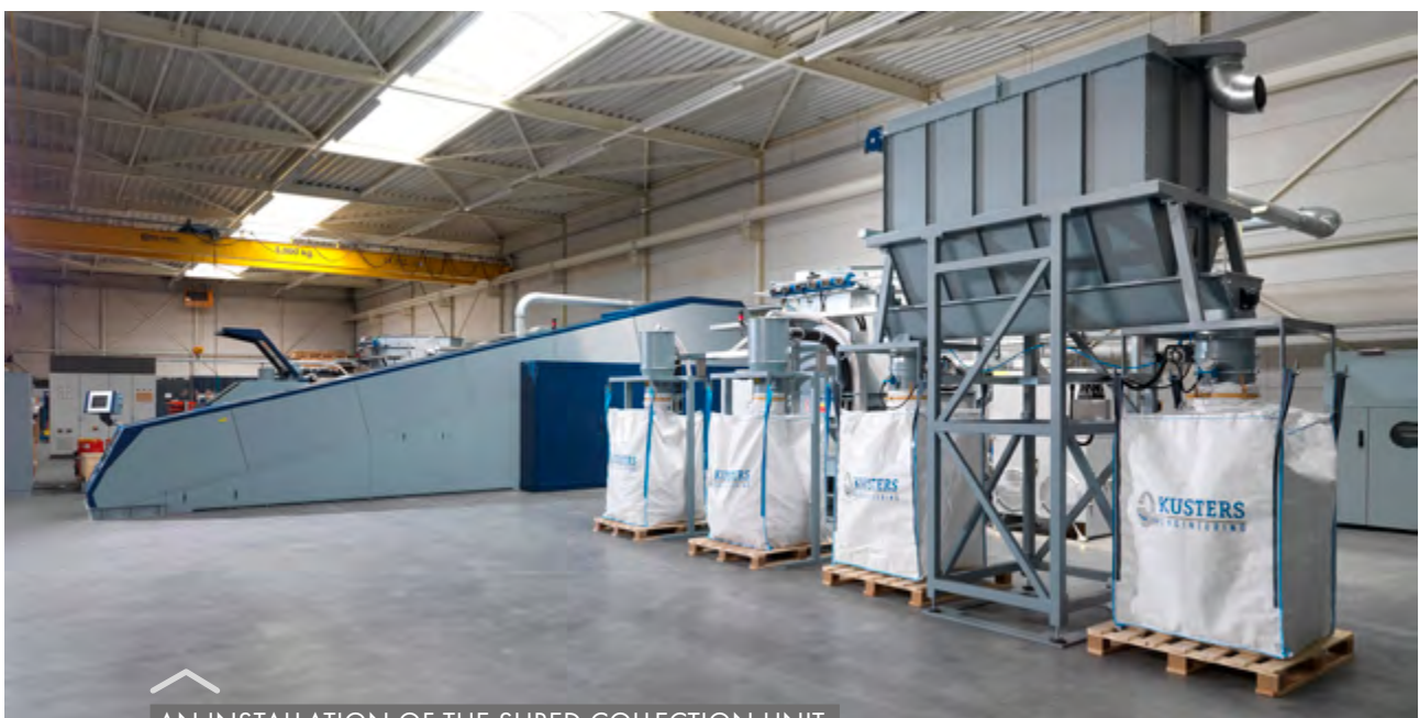
AN INSTALLATION OF THE SHRED COLLECTION UNIT, WHICH RUNS COMPLETELY AUTOMATIC
