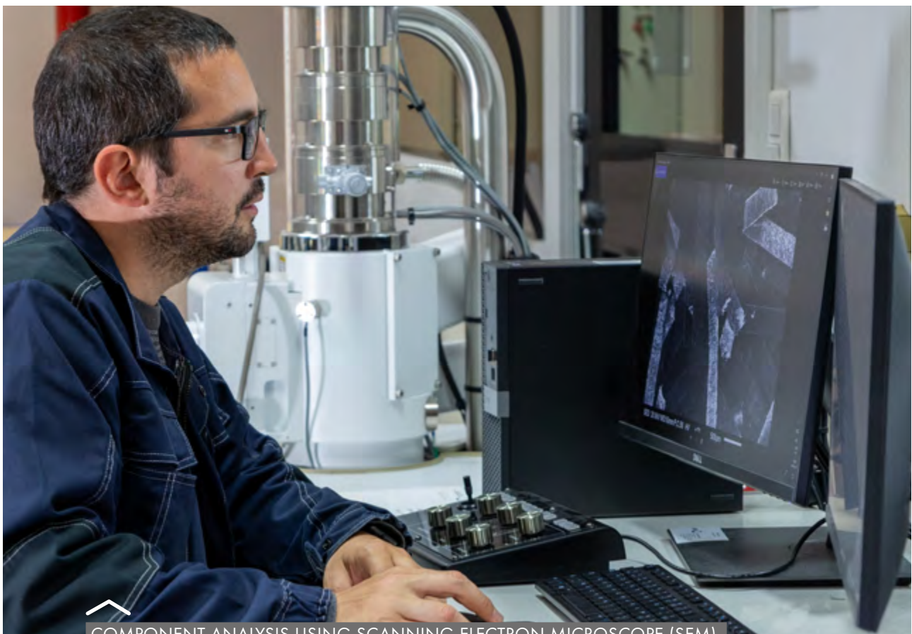
COMPONENT ANALYSIS USING SCANNING ELECTRON MICROSCOPE (SEM).
