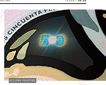
The SET printed lenses work in conjunction with the Clarity<sup>™</sup> C polymer core film offering high levels of optical clarity and careful control of thickness, as well as a gravure printed image to create a feature that is fully integrated with the substrate. Indeed, the feature needs all three elements of lens, film and gravure print to offer the necessary control in order for it to properly work.
