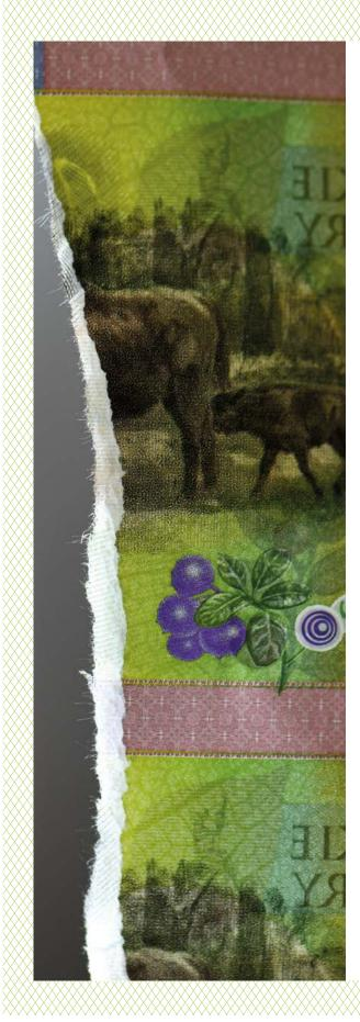
Local atmospheric conditions constitute the first criterion for selecting the substrate for printing banknotes in a given country. Classic paper would be too fragile and more susceptible to mechanical damage (tears) in countries with high air humidity. In such conditions, the priority was, therefore, to increase the mechanical strength of the paper, e.g. by adding synthetic fibres to the pulp as well as to protect the surface against soiling by applying a layer of varnish.
