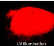
Red emitting phosphour for this specific application has resulted in a colourless, very bright, lightfast (L>5), red phosphor particularly suitable for UV LED excitation.
