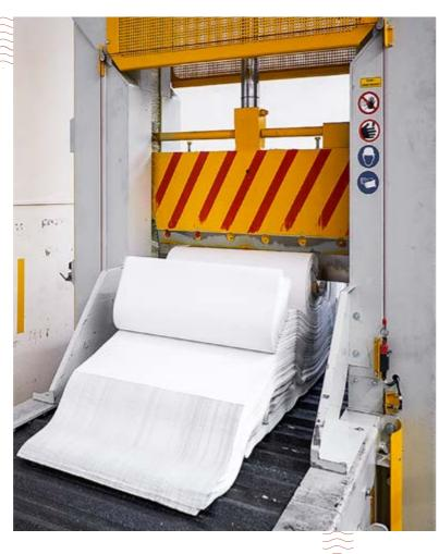
machines is not sent to the shredder but trans- ported in the other direction to the waste container. This high-quality material is re-used in stock preparation. And because the material is pre-shredded, it disintegrates in the pulper relatively quickly.
