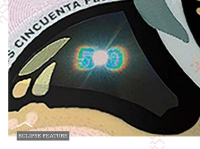
The SET printed lenses work in conjunction with the Clarity  $^{\text{TM}}$  C polymer core film offering high levels of optical clarity and careful control of thickness, as well as a gravure printed image to create a feature that is fully integrated with the substrate. Indeed, the feature needs all three elements of lens, film and gravure print to offer the necessary control in order for it to properly work.
