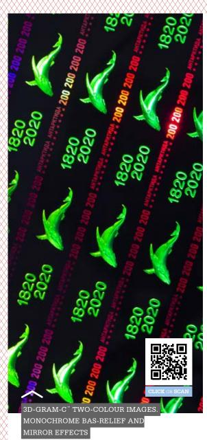
The security stripe on the "Antarctica 200 3D" banknote includes a photopolymer layer with colour images made by 3D-Gram-C<sup>™</sup> (Colour) technology in two contrasting colours - green and red. Stable intense colours, high angular, and spectral selectivity are the main advantages and differences between photopolymer elements and conventional, widespread rainbow holograms.
