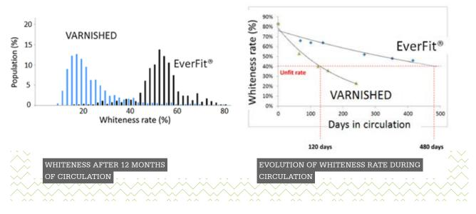
The picture below shows banknotes' resistance to ink abrasion provided by EverFit<sup>®</sup>. As the printed elements are beneath the unprinted laminating film, they are totally protected from abrasion.
